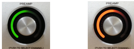
Apollo's hardware preamp knob during normal operation (left) and when a Unison plug-in is in the Unison insert of Apollo's selected channel (right)
