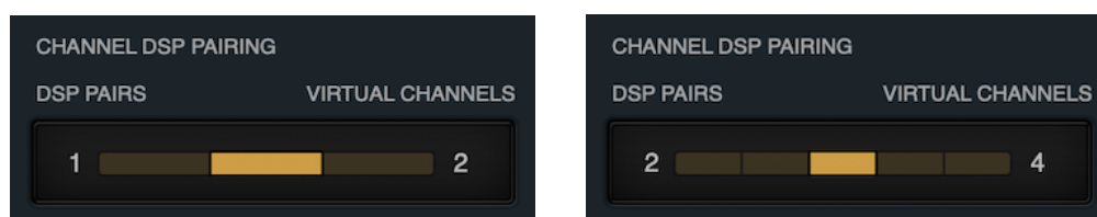
Channel DSP Pairing control as it appears with Apollo Twin (left) and Apollo rackmount models (right)
